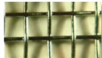
Used for heavy-duty applications in terms of mechanical strength and temperature. Used in suction filters to minimize pressure drop.
